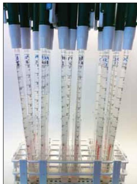
Figure 2. Volumeters used to measure volumes of CO<sub>2</sub> produced by yeast treatments.
